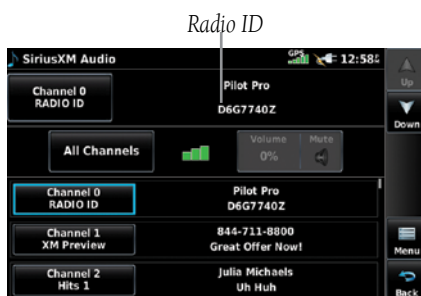
Accessing the SiriusXM Radio ID (Channel 0)
